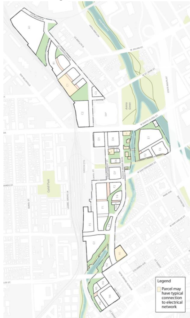
Figure 9.7. Locations of buildings which may be provided with power from PG&E directly instead of the CUP and microgrid.
